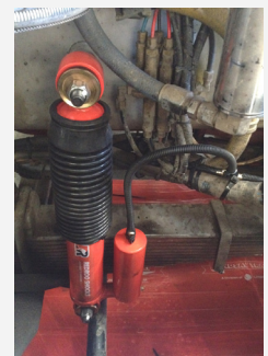
FIGURE 5: 'T' branch and LHS Steer shock.
